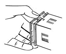
The following switches must be set: the temperature sensor selector, the operating mode selector, and the alarm mode selector. There is also a protection switch that can be set to protect settings. The following figure shows the locations of internal switches on the internal mechanism.
