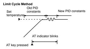
The optimum PID constants are calculated by this method by varying the control output variable and generating external oscillation.
