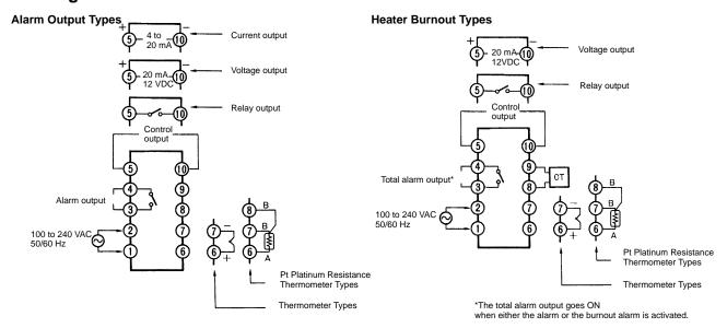
**Note:** Ground FG terminal 18 to avoid ambient noise. Do not connect unused terminals.
