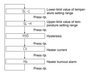
Of the above parameters, only the hysteresis, which is described below, differs from the parameters for PID control. Refer to 1. PID Control for details on other parameters.
